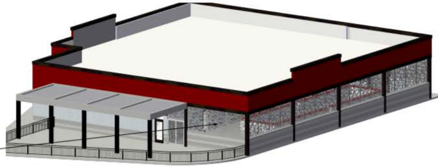
Perforated metal panels @ exterior bar walls
